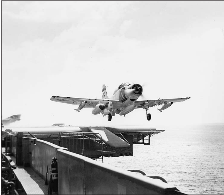
A Zappers EA-1F Spad, outfitted with two ALT-2 jammers on the outboard wing stations, an APS-31 radar pod on the right inboard station and a centerline fuel tank, leaps from Constellation's (CVA-64) waist catapult, Aug '67.
