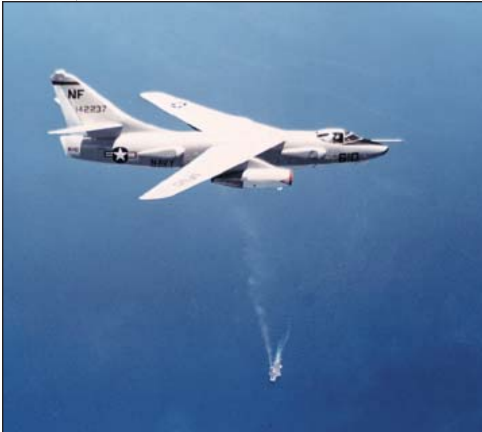
Left: EKA-3B Skywarrior at sea with CVW-5/ Midway (CVA-41), c. 1970. The blisters on the side of the aircraft contain transmitter antennae for the ALQ-92 VHF jamming system. Left, below: A pod of Whales on the ramp at NAS Alameda, 1969. The first three aircraft, all EKA-3Bs, were assigned to USS Oriskany's (CVA-34) Det 34 and will receive CVW-19's "NM" tailcode as they embark. The fuselage stripes indicate the first, second and third det aircraft, useful to help identify specific tankers when large gaggles of strike aircraft take fuel. The aircraft on the far right is a KA-3B.
